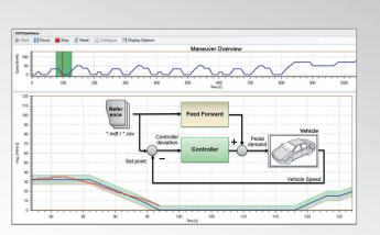
To increase vehicle testing and calibration efficiency, FEV has developed TOPEXPERT VTA. It facilitates the calibration engineer to plan test sequences at the desk using a comfortable graphical maneuver editor. The generated test descriptions can be executed in the vehicle, either guiding the engineer through the maneuver or completely taking over vehicle control. By this, testing time is reduced and test reproducibility and data quality is significantly enhanced.
