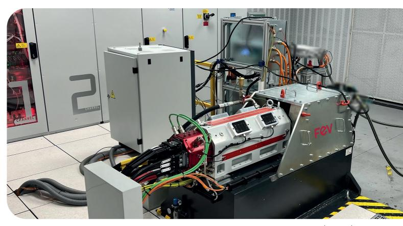
Dynamic E-Motor test bench of 24 000 rpm and above: good accuracy for speed control for low speed (0...10 rpm)
